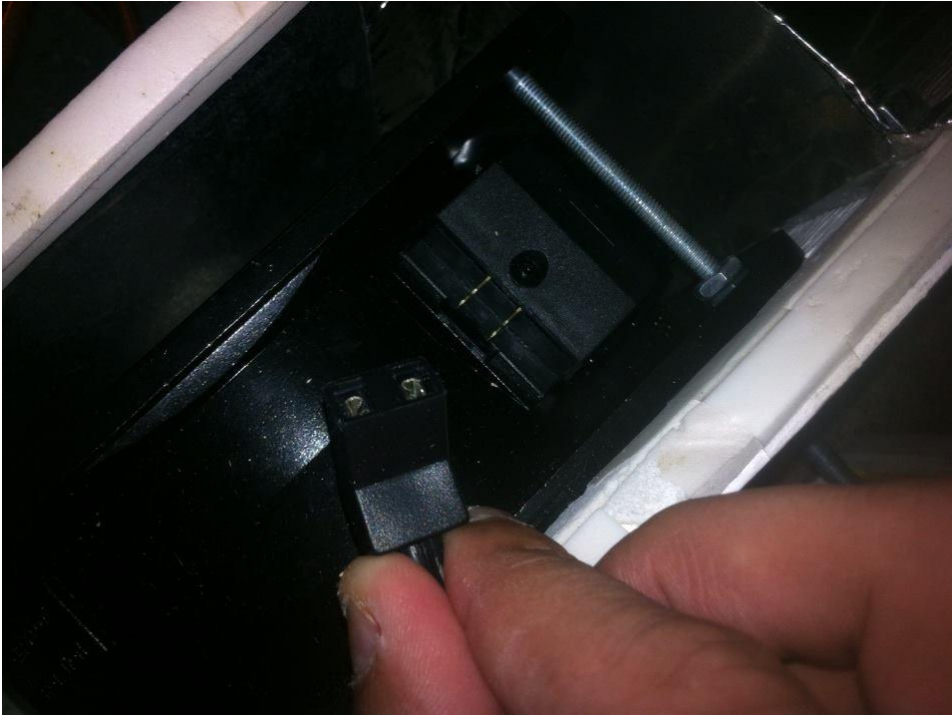
Figure 10: Fan Electrical Connection
