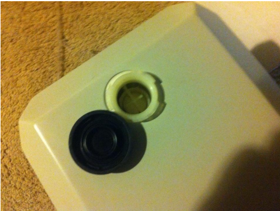
Figure 11: Chiller Process Fluid Tank Access
