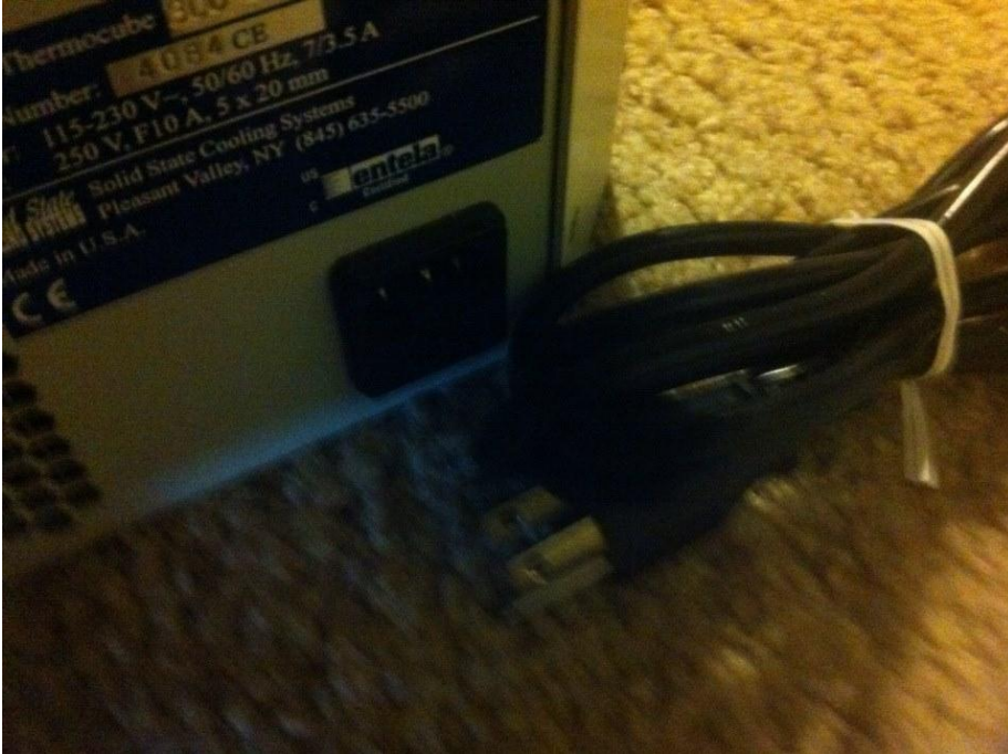
Figure 13: Chiller Power Cord and Connection
